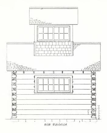
Figure 56. Log lookout house, Plan L-3. This illustration was drafted in 1928 for the Northern District. It is only a portion of the plan sheets for this structure. As with the other Figures in this series (54 through 70) only one representative view or other interesting detail was selected from each set of plans.
